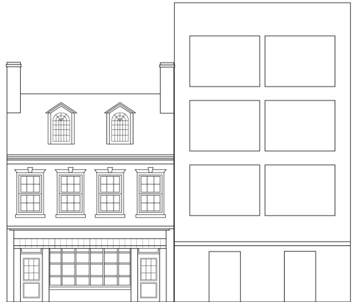
ADDITION WITH INAPPROPRIATE SCALE AND FENESTRATION
